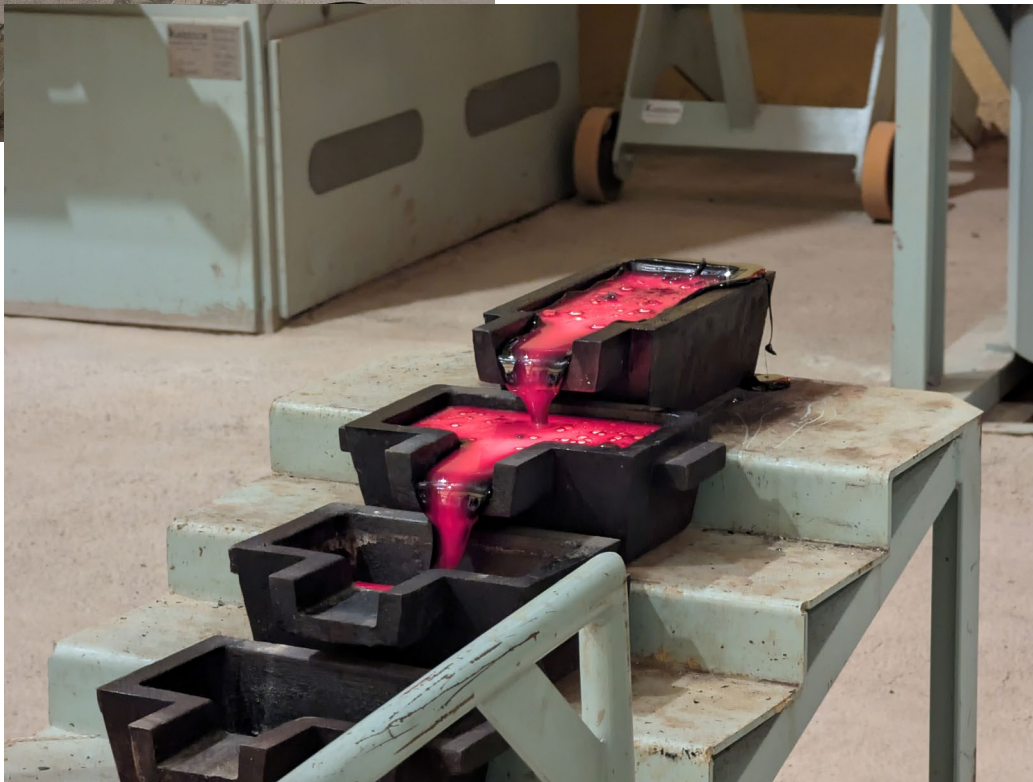
Red-hot smelted concentrate
