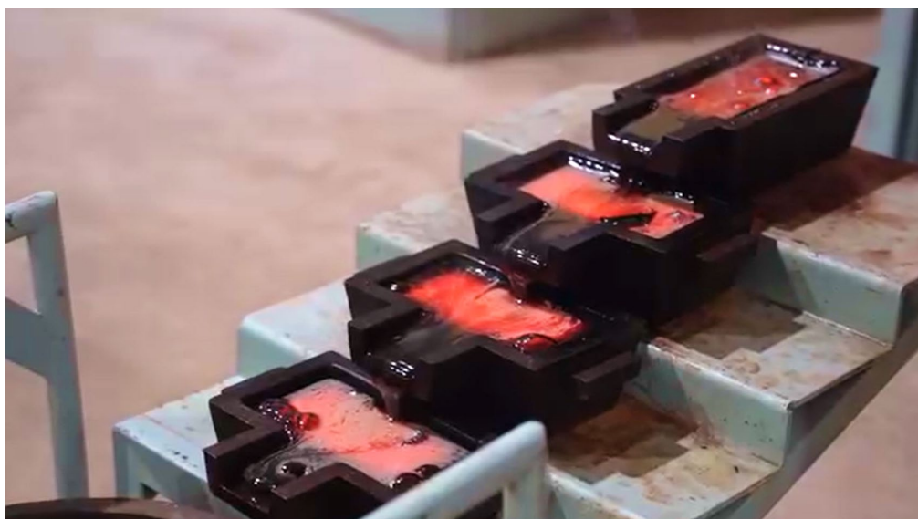
The red-hot poured smelt from the oven
