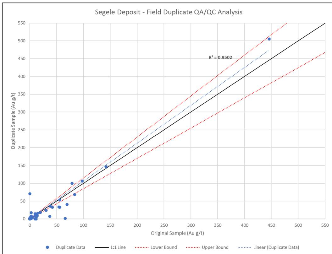
**Figure 5-4: Diamond drilling field duplicate HARD plot**
