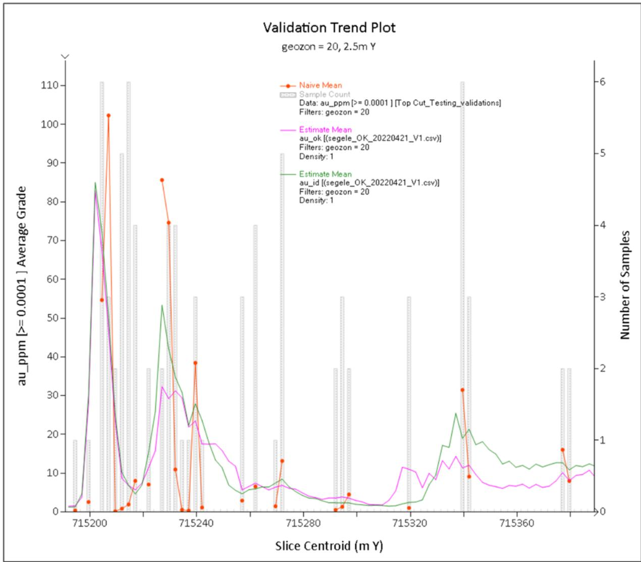
Figure 8-9: Elevation swath plot for domain geozon – 20 (footwall lens 1)
