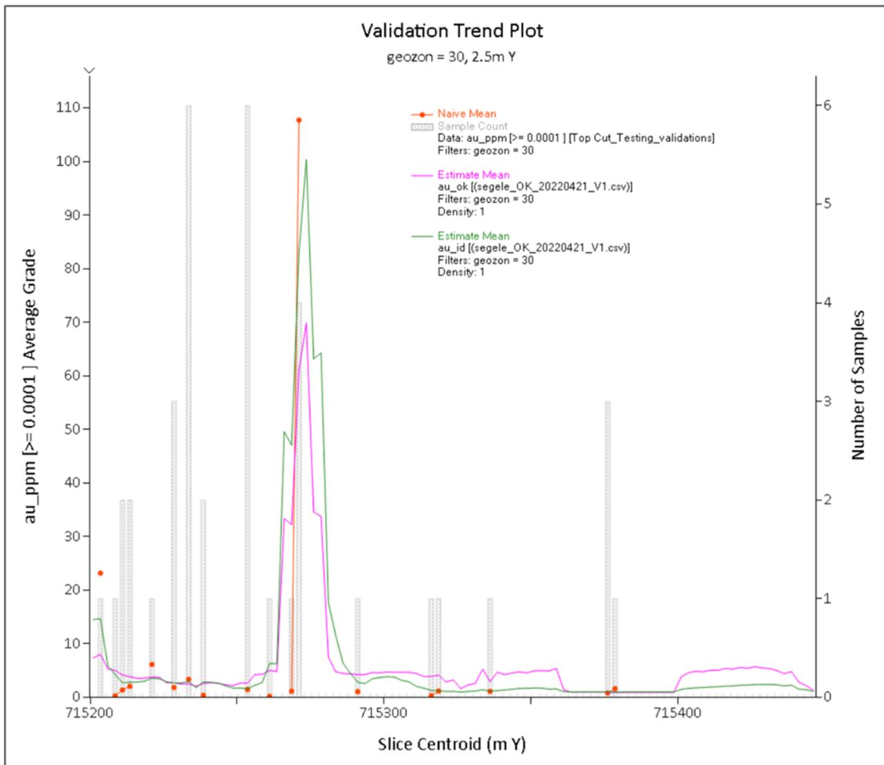
**Figure 8-12: Elevation swath plot for domain geozon = 30 (footwall lens 2)**
