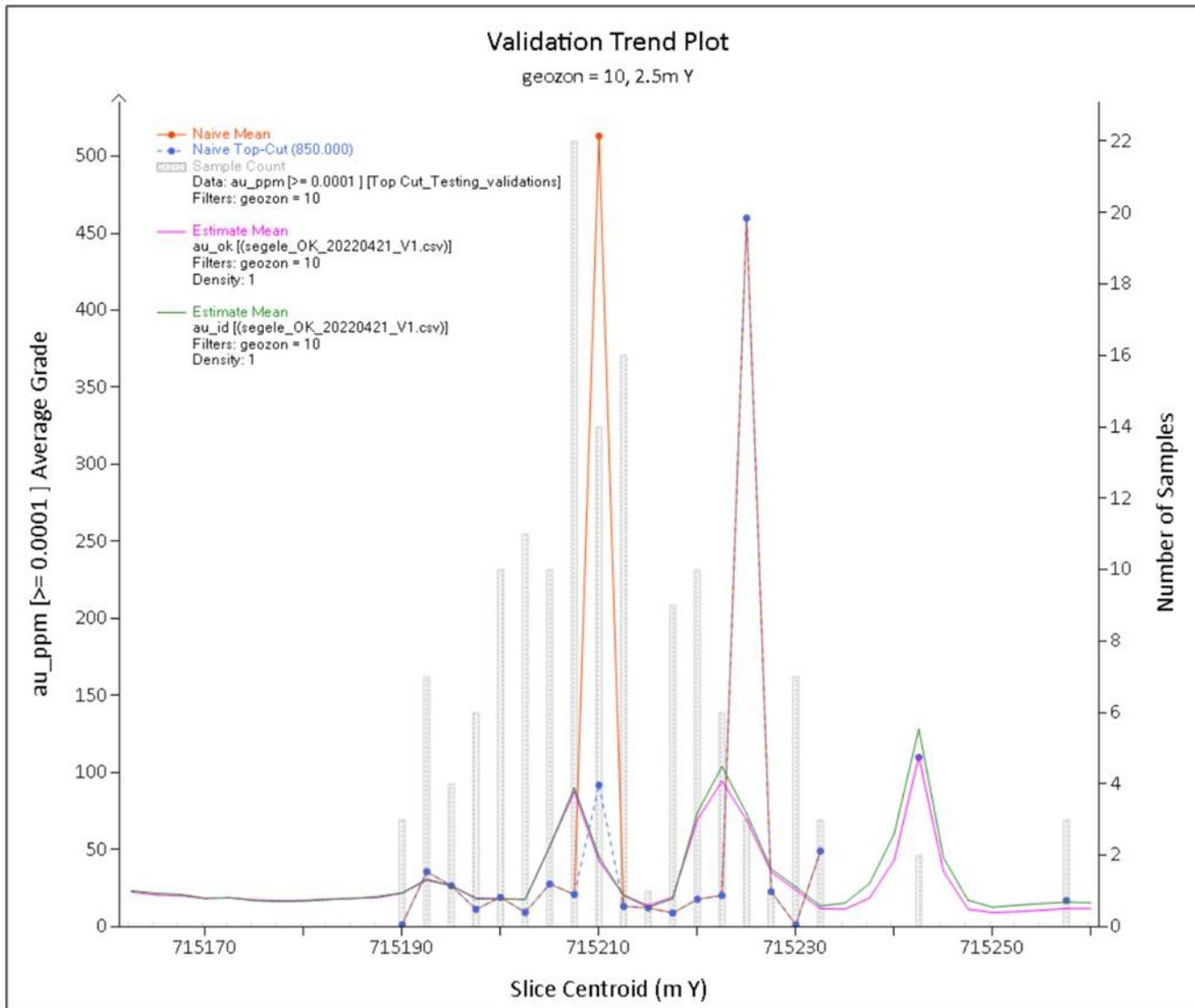
Figure 8-6: Elevation swath plot for domain geozon = 10 (main lens)
