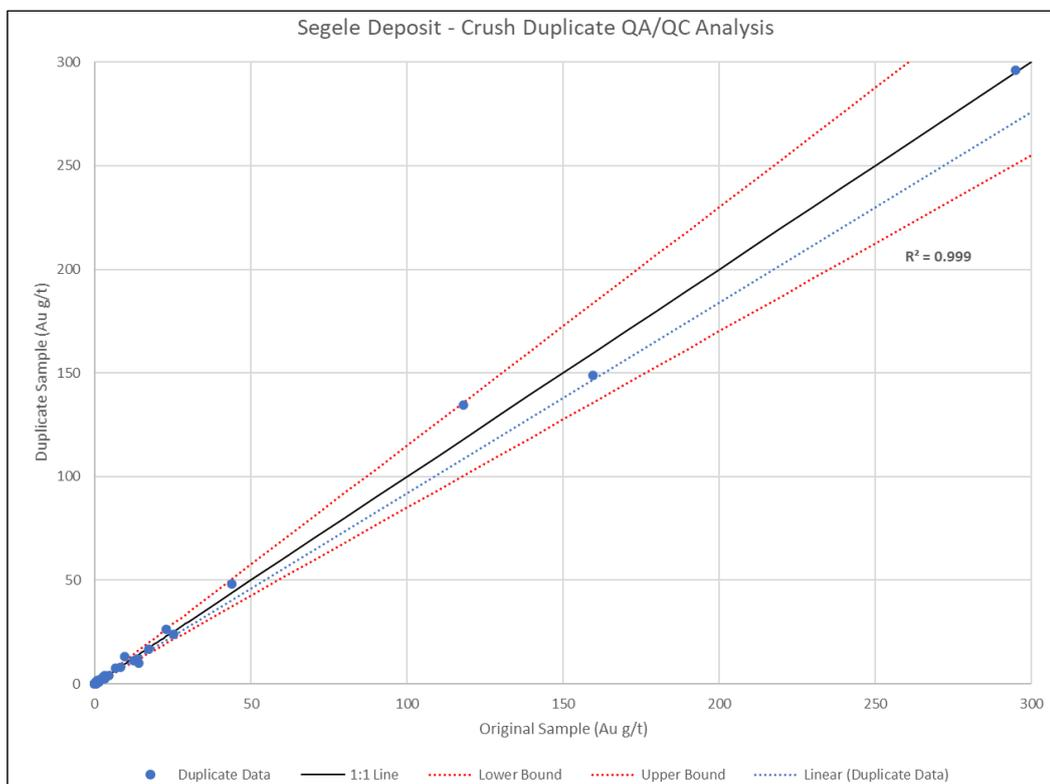
**Figure 5-10: Scatter plot of original versus laboratory crush duplicate samples**
