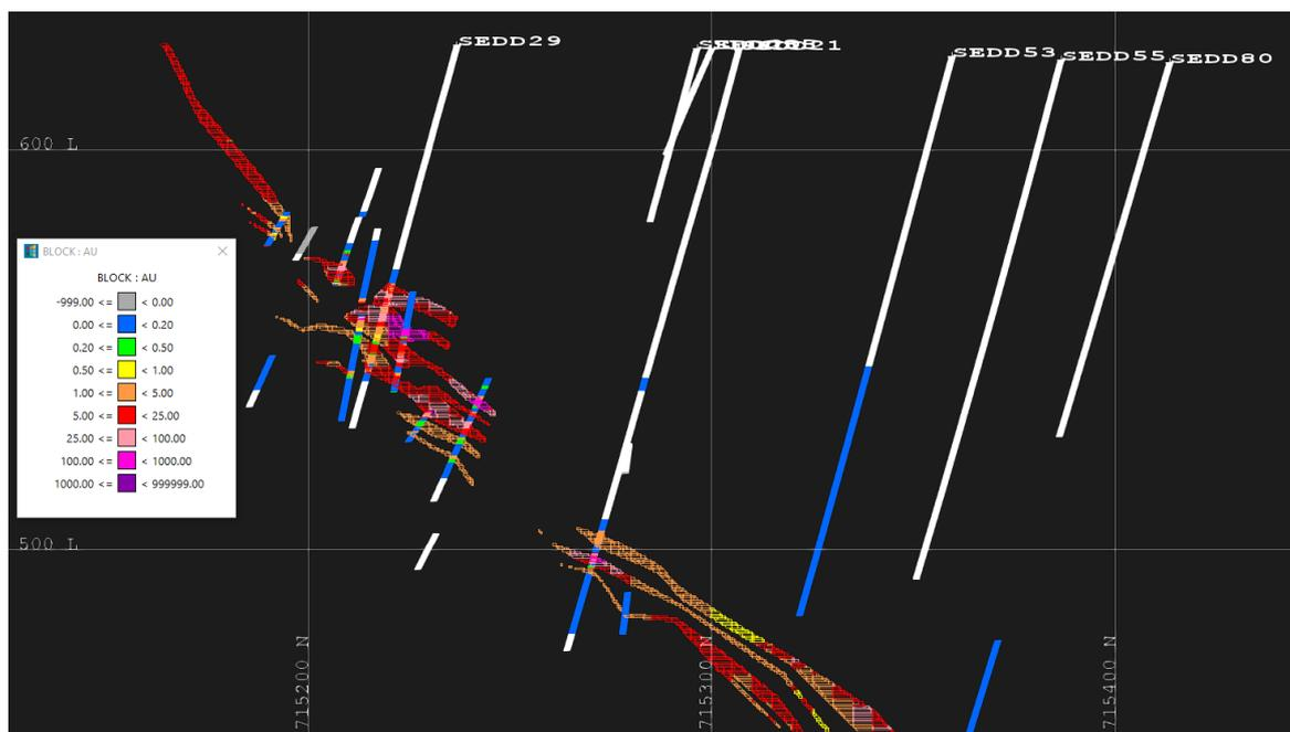
**Figure 8-2: North–south cross section 727,540 mE looking west showing mineralised lens 20, 30 and 40**
