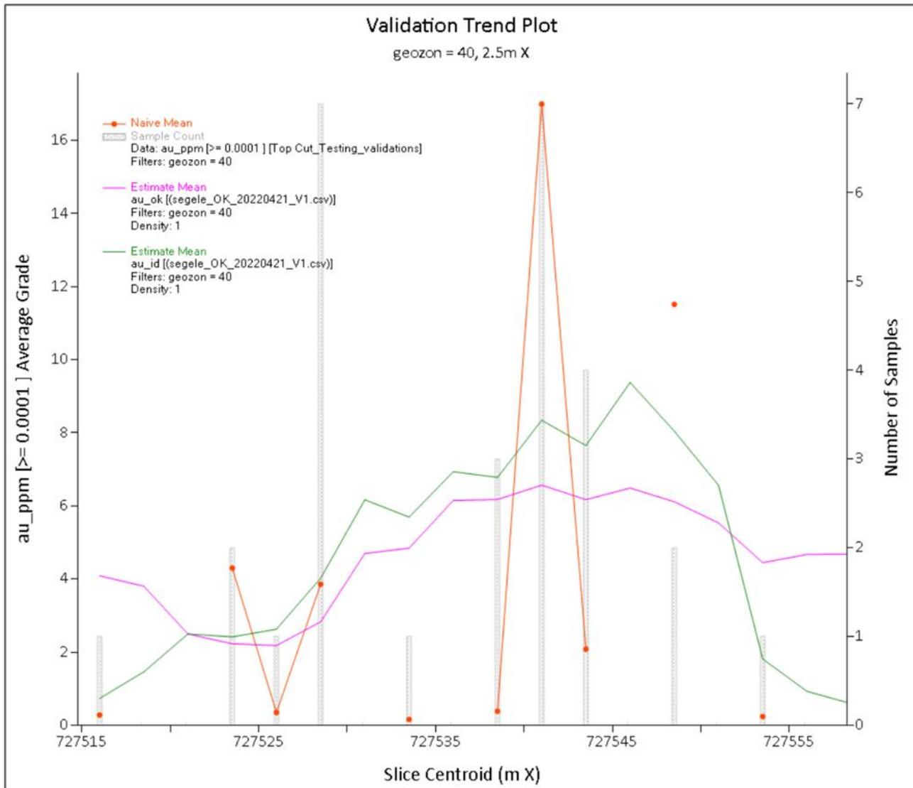
Figure 8-14: South to north swath plot for domain geozon = 40 (footwall lens 3)
