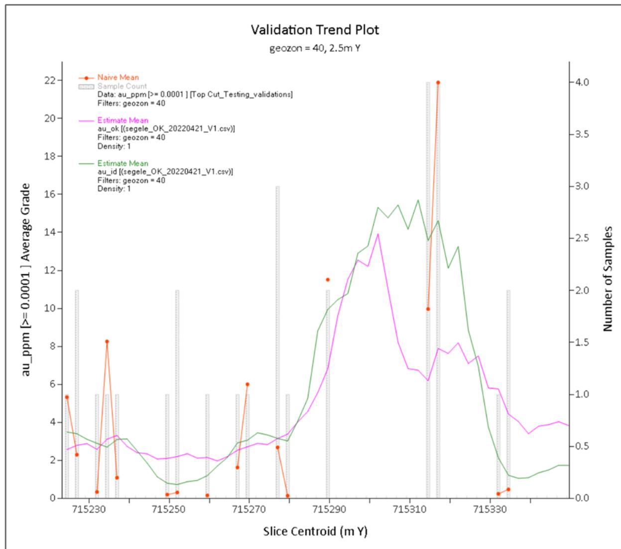
Figure 8-15: Elevation swath plot for domain geozon = 40 (footwall lens 3)
