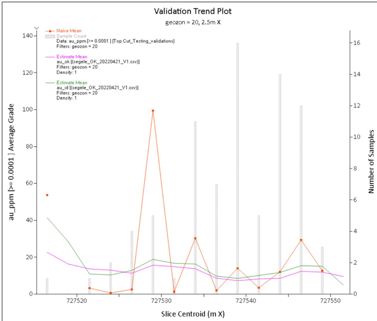
Figure 8-8: South to north swath plot for domain geozon = 20 (footwall lens 1)
