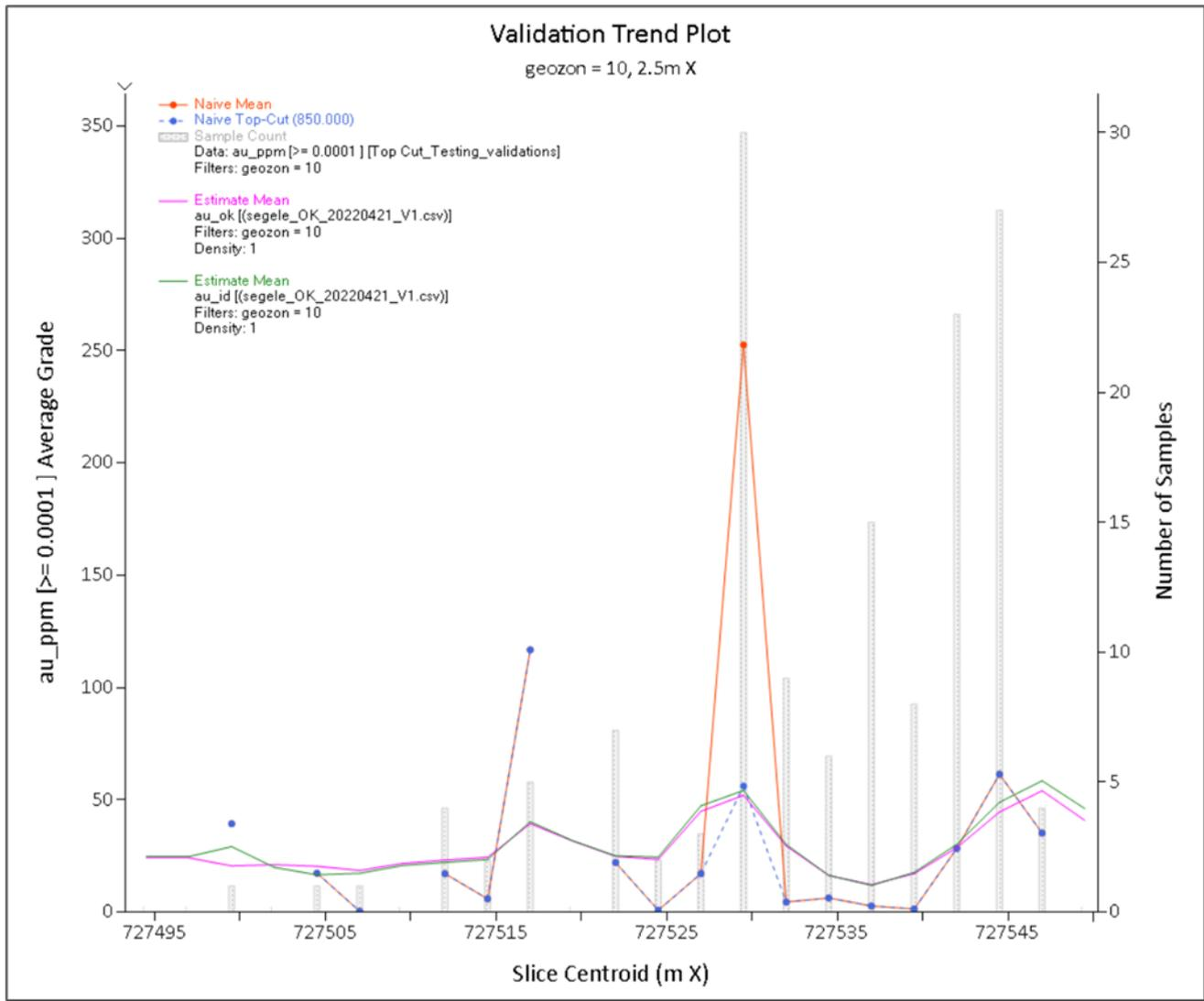
**Figure 8-5: South to north swath plot for domain geozon = 10 (main lens)**
