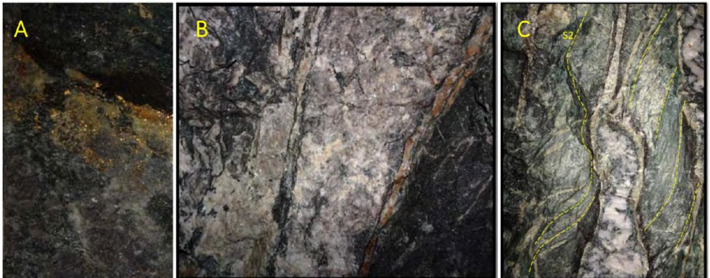
Figure 10: Mineralisation and structure from of the Pahtavaara Deposit. A: Free gold in drill core. B/C: Polyphase structures and veining.
